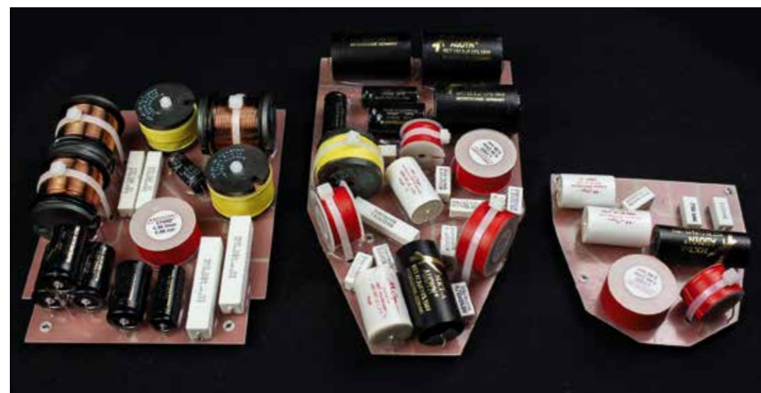
◀ For each frequency range, the Gauder has its own crossover equipped with highest quality components from Mundorf.
